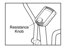
decrease the resistance, turn the knob counterclockwise. Important: The knob may not stop turning when maximum or minimum resistance is reached. When the knob becomes more difficult to turn, stop turning it or damage will result.
